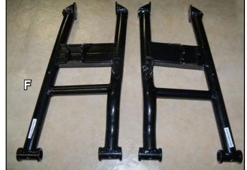
This product is designed, and manufactured, to gain additional ground clearance on utility vehicles and to be used at slower speeds on level terrains. Installation of this product increases angle of Axles which may result in frequency of required maintenance and parts wear. It is recommend that wider Tires or Wheel Spacers be used, in conjunction, with this kit to improve stability.
